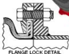
FLANGE LOCK DETAIL
